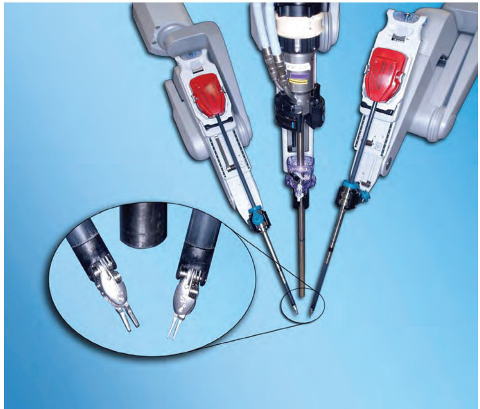
Figure 25.3 Robotic laparoscope and two robotic arms with robotic instruments inserted. The tip of the instruments can be appreciated in the insert.
