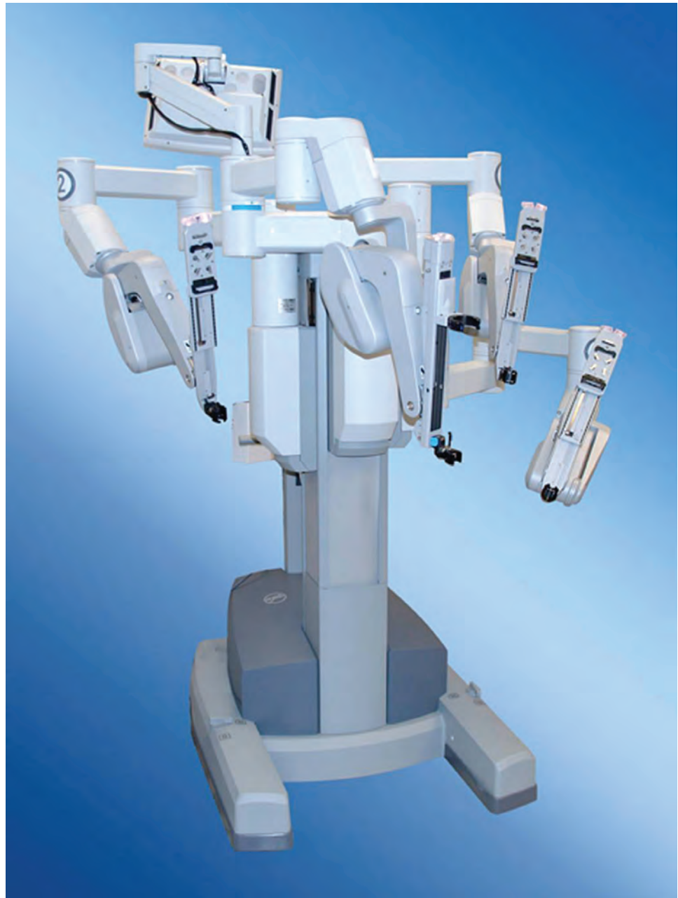
Figure 25.1 Robotic column with robotic arms.
