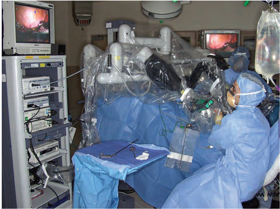
Figure 25.6 The robotic column is usually positioned between the patient legs for pelvic surgery. The assistant is seated to the left of the patient and is scrubbed for the procedure.
